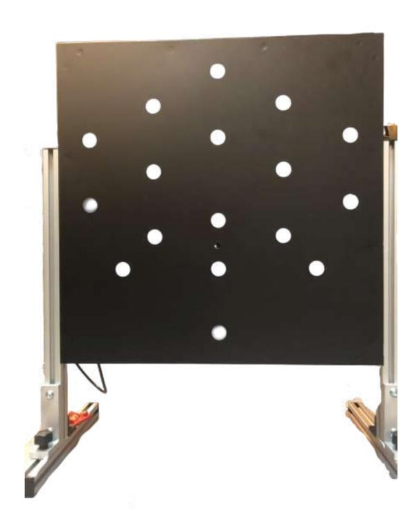
The PAC Matrix (Matrix of sensors for Photometric Airfield Calibration) is a **portable photometry measurement system that can be used both in workshop** and on-site.
